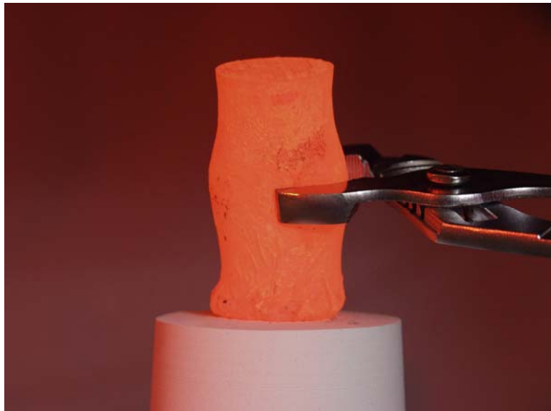
Figure 1: 1-inch diameter copper alloy semi-solid billet being squeezed by an adjustable pliers at 50% solid/50% liquid. This SSM material has the consistency of modeling clay.
